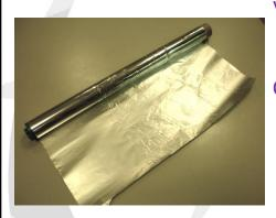
Vary in thickness from 11 micron up to 14 microns
