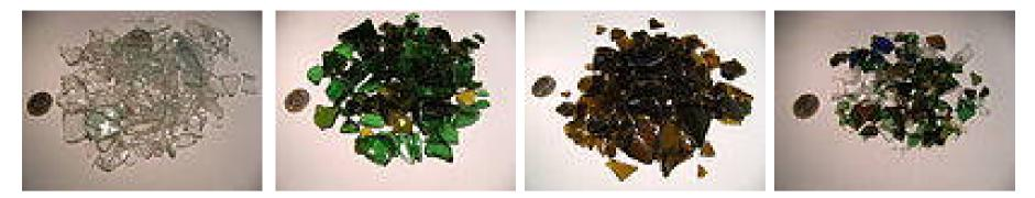
Glass that is crushed and ready to be remelted is called **cullet**. In addition to the mineral ingredients, a glass batch traditionally consists of 25 to 90 percent cullet. Cullet is crushed rejected glass, generally of the same composition as the mineral mixture, that is included because its early melting in the furnace brings the mineral particles together, resulting in accelerated reactions. In average 64% of glass produced in Europe is made of recycled glass.
