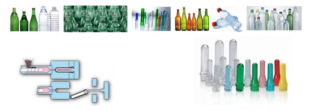
The process is simple, the heated PET which is in the molten form is injected into the injection chamber, by the rotation of screw barrel within the machine, until the chamber is full.
