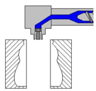
Same as PET bottles, polycarbonate items starts as a resin. It needs to be injected into the mould via a nozzle or tube, depending upon the application, and cooled to make the mold solid. The injection moulding process happens between 280 – 320 °C.
